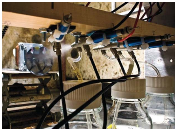
Figure 4. Photograph of simple automated spray-LbL laboratory setup illustrating the coating of a silicon wafer.
